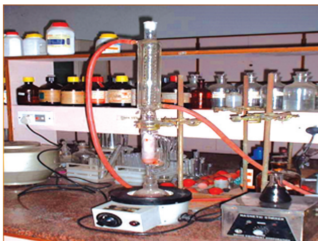
Figure 92: Solvent extraction unit
