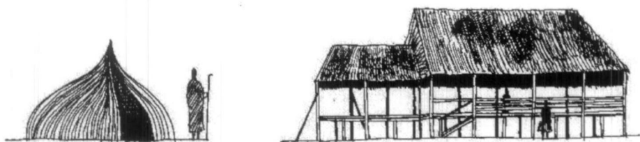
FIG. 2.6. Two examples from the great range of house forms using thatch and wood as materials. Left: Masai dwelling (Africa). Right: Yagua dwelling (Amazon). The houses in figures 2.3 through 2.6 are not drawn to the same scale, but their size is indicated by comparison with the human figure.
