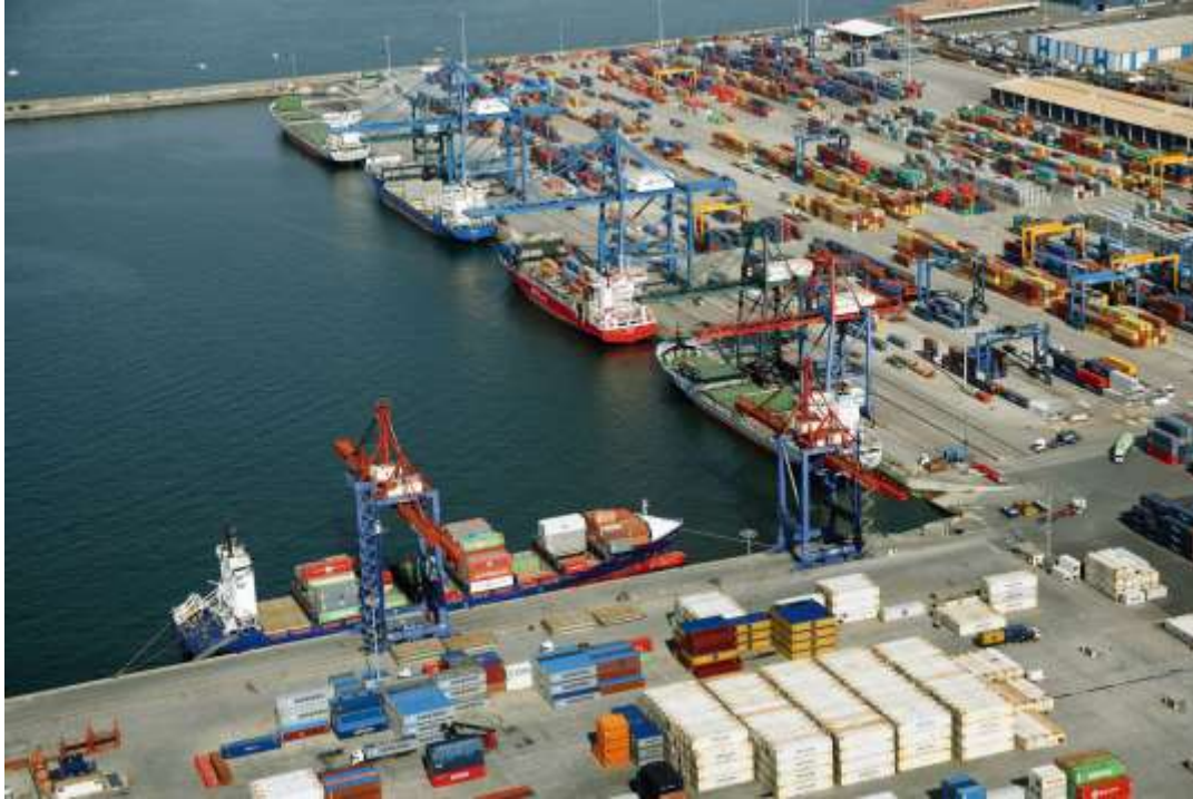
Figure 2.15-4: Discrete Berthing Layout
