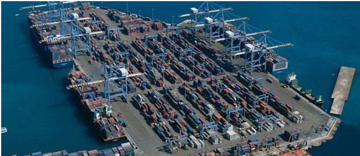
Figure 2.15-3: Indented berthing layout, Port of Busan, South Korea
