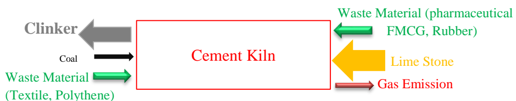
Figure 5-Waste Co Processing while Clinker Manufacturing
