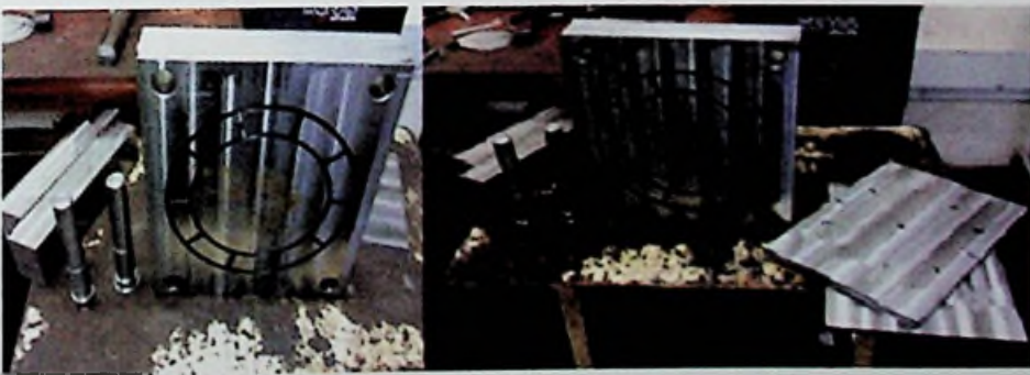
Figure 56 Injection mold under manufacturing
