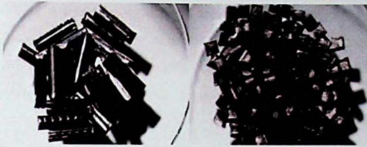
Figure 49 Nylon short glass fiber vs. long glass fibers (66)
