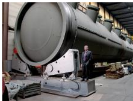
Figure 9: PEMA welding mounts automated
