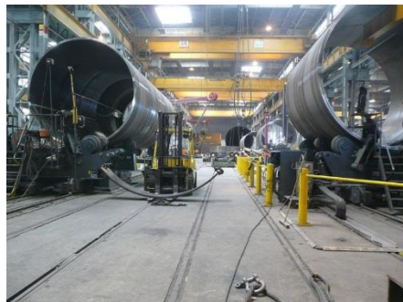
Figure 8: PEMA welding Mounts
