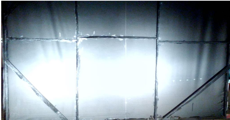
Figure 3-14 Light distribution of Test No 2, Scattered beam due to poor aiming
