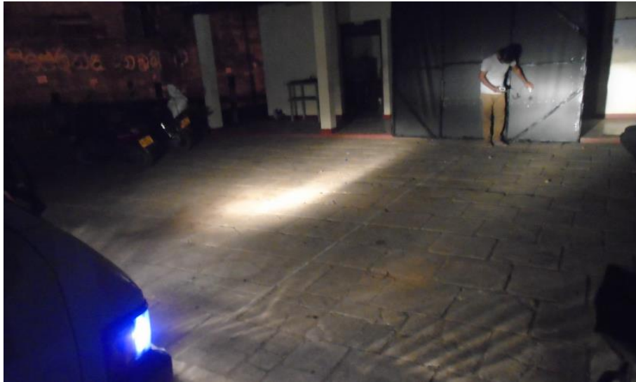
Figure 3-16 Light distribution of Test No 9, Very Poor Illuminance intensity and Very Poor aiming, Recently faced with an accident.
