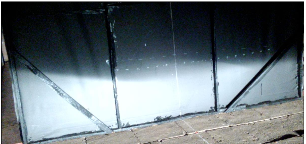
Figure 3-9 Photograph of low beam operation Test No:4 , The cutoff line is slightly unclear and illuminance intensity is low by visual inspection.
