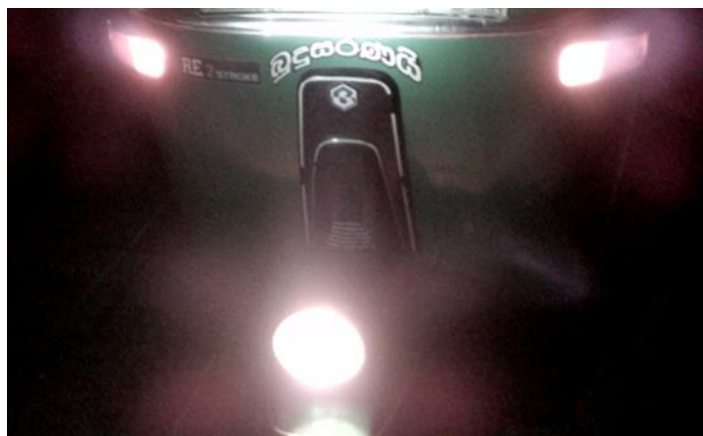
Figure 3-16 Light distribution of Test No 9, Very Poor Illuminance intensity and Very Poor aiming, Recently faced with an accident.
