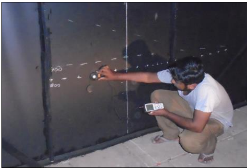
Figure 3-6 Measuring illuminance intensities using Lux meter
