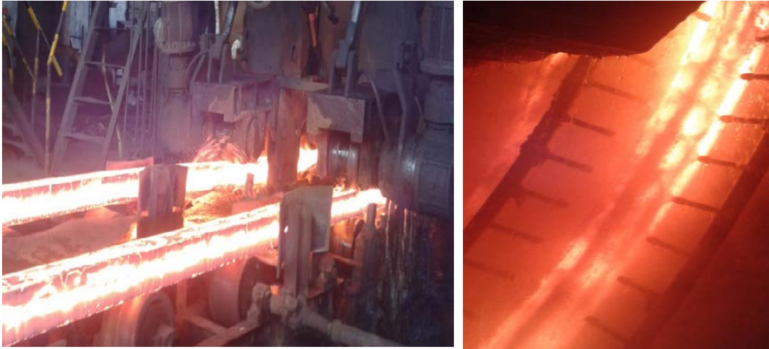
Figure 2.8: Photographs of the continuous casting of billets
