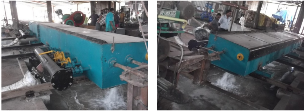
Figure 3.2: Photographs of the water quenching process
