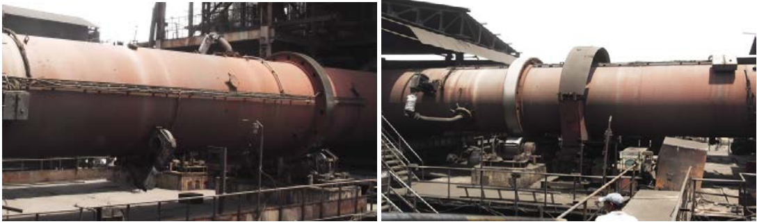
Figure 2.5: Photographs of the horizontal Kiln used to manufacture sponge iron
