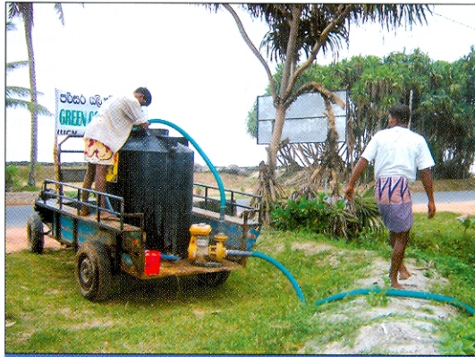
A Hand Tractor with a Tank and a Pump was Used for Watering
