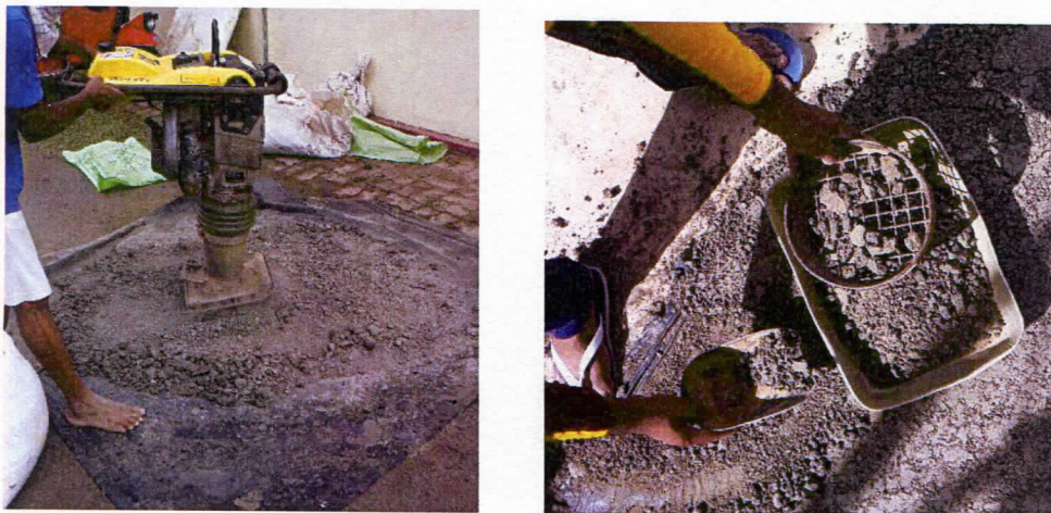
Figure 6.1 Crushing and sieving Murunkan soil
