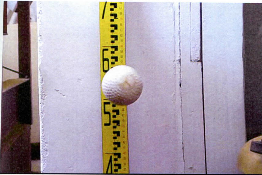
Figure 5.23 Image of the ball at its maximum rebound height (MU day 3)
