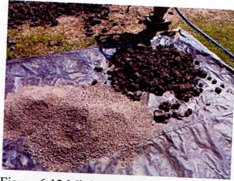
Figure 6.13 Mixing of two soils
