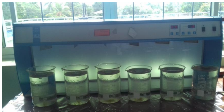
Figure3.5: Photograph Showing the Flocc Settlement at Different Dose of Coagulants Using Jar Test Apparatus
