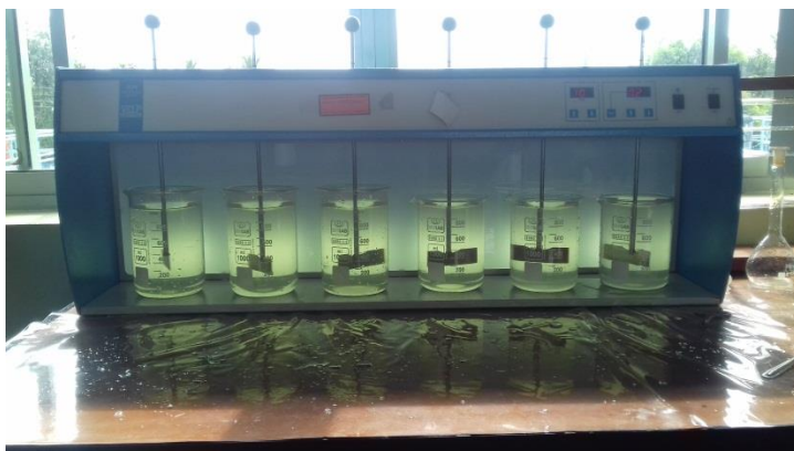
Figure3.4: Photograph Showing the Flocc formation at Different Dose of Coagulants Using Jar Test Apparatus
