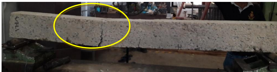
Figure 4.3: Failure mechanism of beam Type F1
