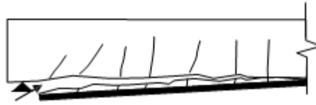
Figure 2.6: CFRP sheet with concrete cover separation (Garden and Hollaway, 1998; Smith and Teng, 2002; Ashour et al, 2004; Esfahani et al, 2007).
