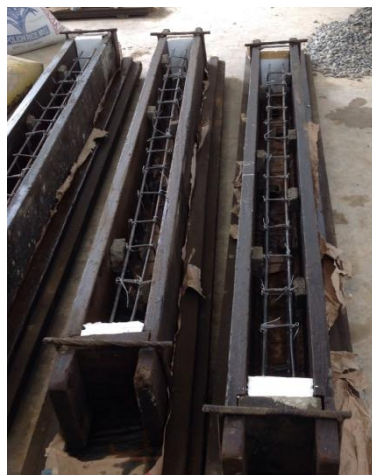
Figure 3.3: Prepared formwork arrangement with R/F cage and casted beam
