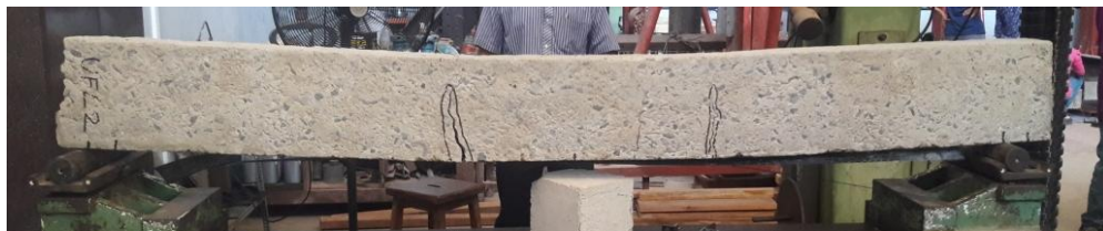
Figure 4.6: Failure mechanism of beam Type F2
