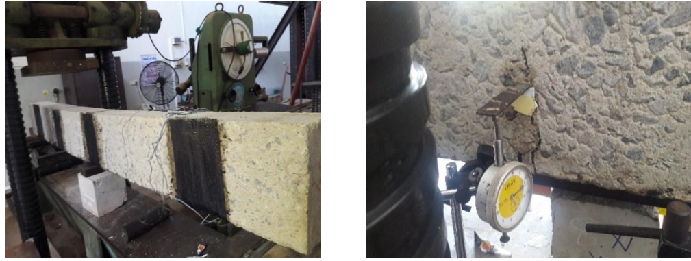
Figure 3.17 : Fixed dial gauge to beam
