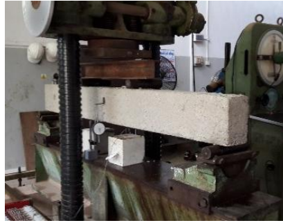
Figure 3.4: Beam testing using Amsler machine
