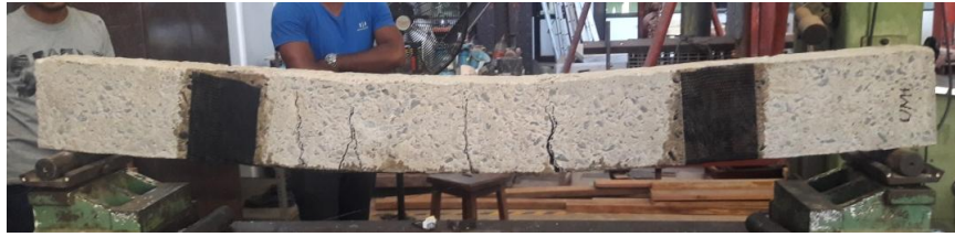
Figure 4.13: Failure mechanism of beam type M1
