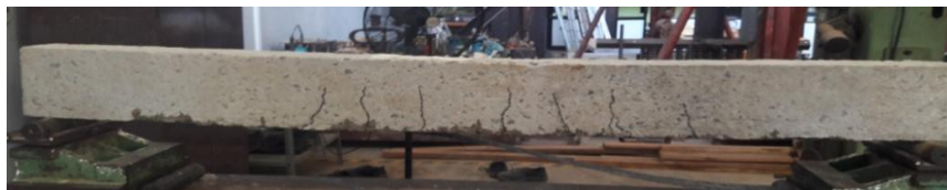
Figure 4.10: Failure Mechanism of beam type “IN 2”
