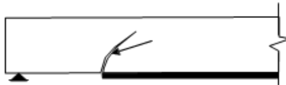
Figure 2.4: Diagonal shear crack at CFRP sheet end (Garden and Hollaway, 1998; Smith and Teng, 2002; Ashour et al, 2004; Esfahani et al, 2007).
