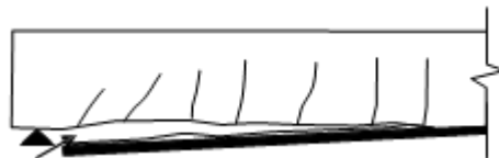
Figure 2.5: CFRP sheet interfacial de-bonding (Garden and Hollaway, 1998; Smith and Teng, 2002; Ashour et al, 2004; Esfahani et al, 2007).
