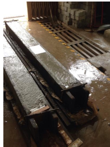
Figure 3.3: Prepared formwork arrangement with R/F cage and casted beam
