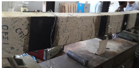
Figure 4.29: CFI1 beam after loading
