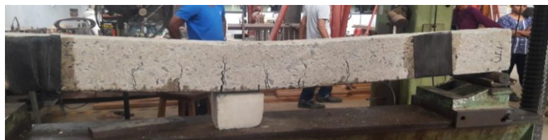
Figure 4.8: Failure Mechanism of beam Type “IN 1”
