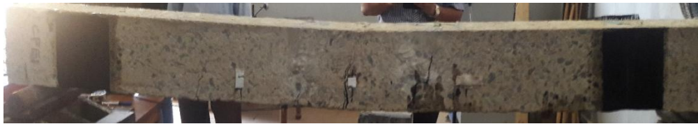
Figure 4.25: CFE1 beam after loading
