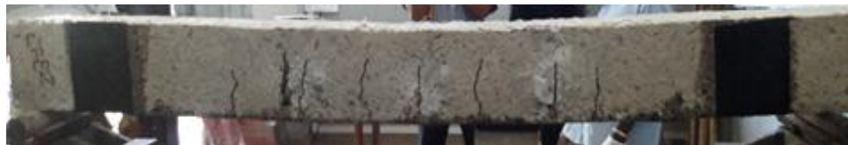
Figure 4.47: Crack distribution of CFRP strengthened pre-cracked beams
