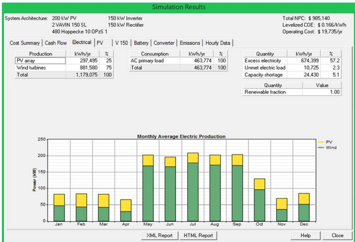
Figure 7.8: Monthly average electricity production for the load profile without ice plants (only with RESs)
