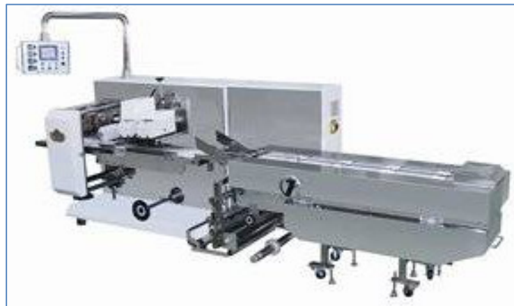
Figure 1.2: Automatic horizontal pillow wrapping machine.
