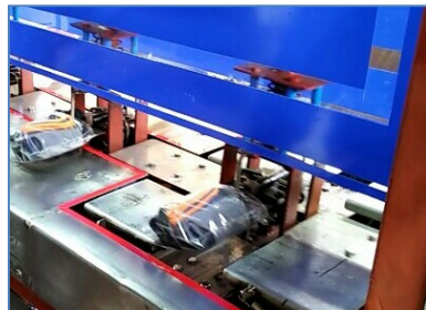
Figure 5.9: Duple plates down and glove pair moves to stripping station
