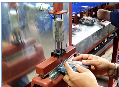
Figure 5.11: Seal the poly bag using auto sealer
