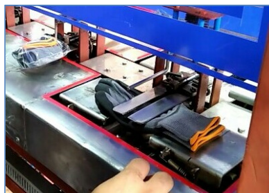
Figure 5.3: Machine releases duple plates down
