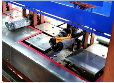
Figure 5.7: Squeeze the glove pair
