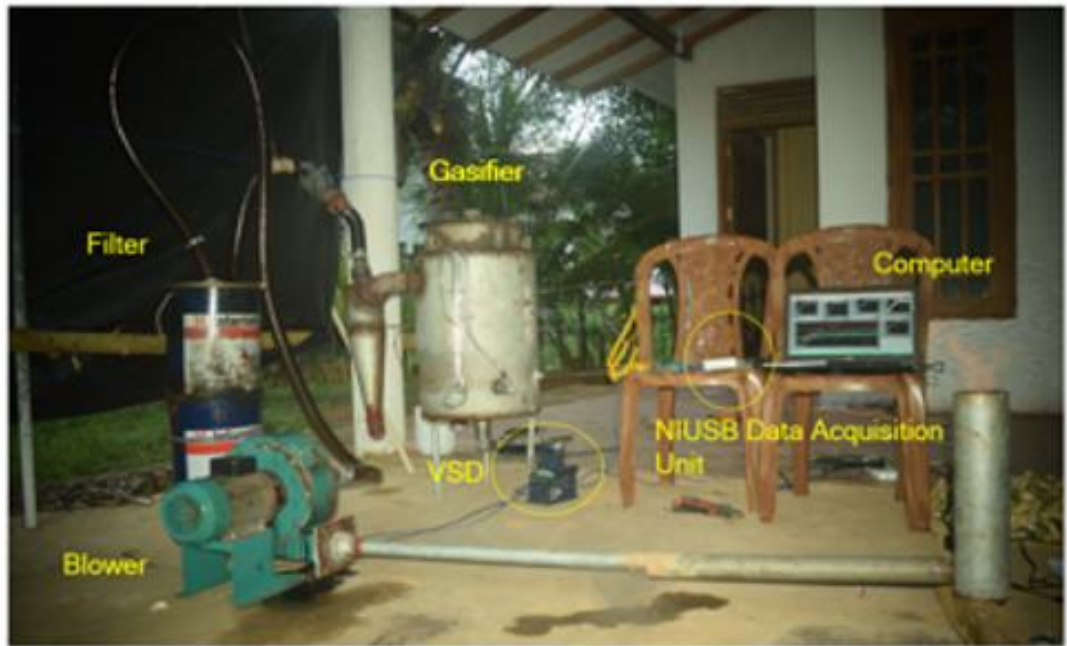
Figure 3. 10: Experimental Set-up of Downdraft Gasfier
