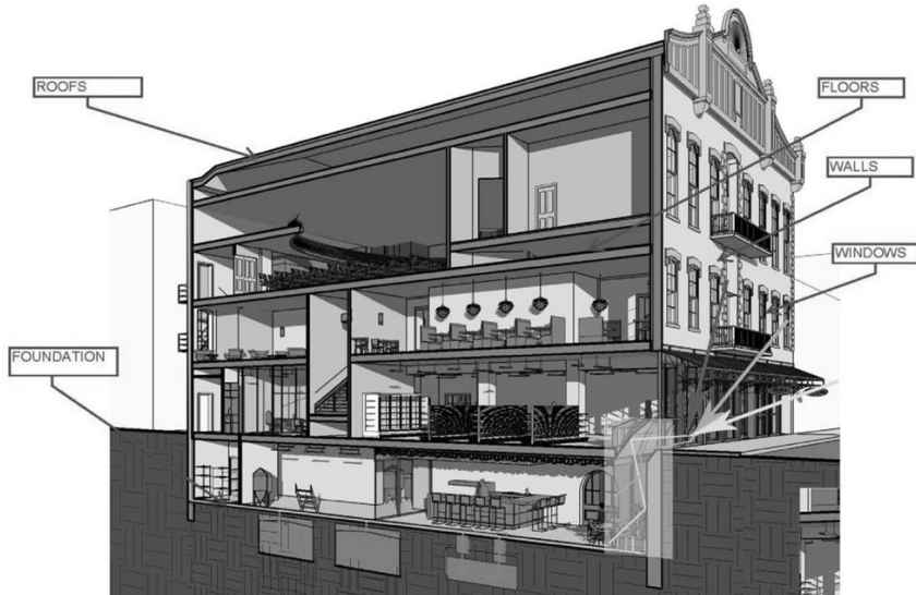
Figure 1 Building Materials and Assemblies included in LCA
