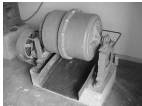
Figure 4, Ball mill to grind the burnt husk
