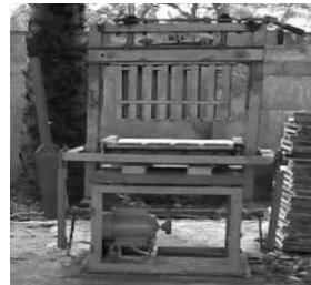
Figure 2, Interlocking block casting Machine
