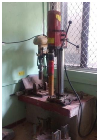
Figure 3.2: Core drilling machine used for core sample preparation
