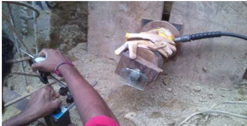
Figure 3.15 Apparatus used to pull the test nails
