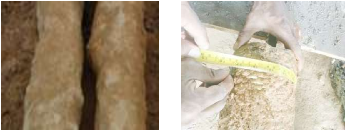
Figure 3.22 Extracted soil nails
