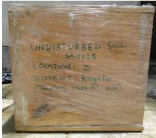
Figure 4.5 Tagged, packed undisturbed soil sample ready to be transported to the lab
