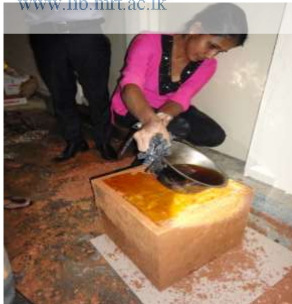
Figure 4.4 Sealing the surface of the undisturbed soil sample
