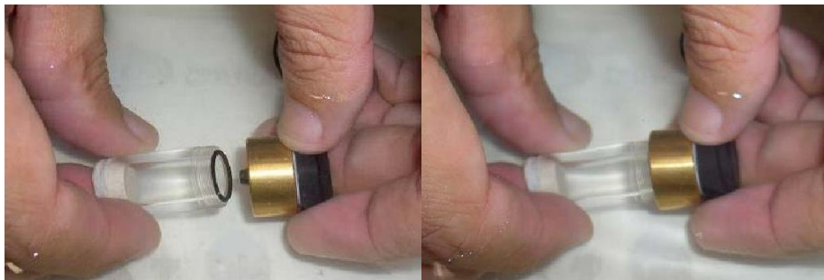
Figure 5.21: Screwing the acrylic tube with O-ring in the sensor body to achieve tight seal
