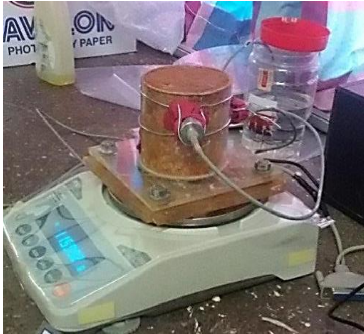
Figure 6.2: Typical arrangement for permeability function test for drying path
