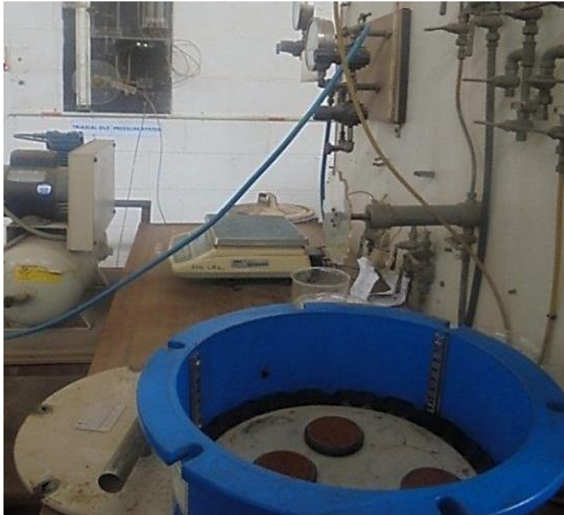
Figure 4.1: Typical arrangement of 5-bar pressure plate apparatus used for the research
