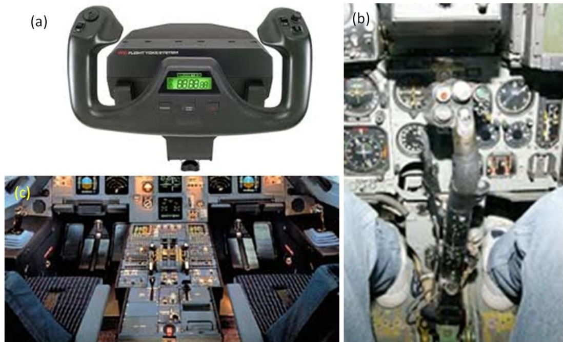
Figure 1.5: (a) Yoke controller, (b) Center stick controller, (c) Side stick controller
