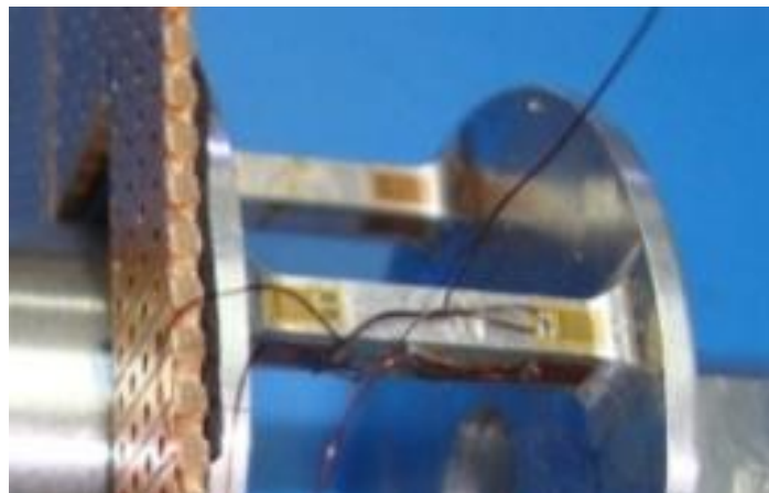
Figure 3.2: Strain gauge placement on single column.
