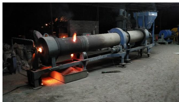
Fig. 01. Lab scale rotary kiln at Datiya, TARAGram
