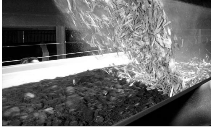
Fig. 2.14 :Mixing Biomass with coal under 1 st Method of Direct Co-firing [1]
