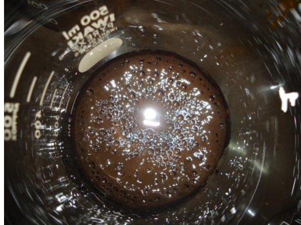
Figure 4.13: Air bubbles trapped at the top of the emulsion sample
