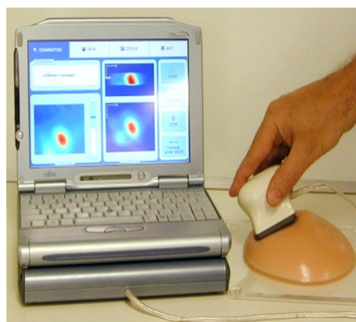
Figure 2.2: General view of breast tactile imager Source: Mechanical Imaging of the Breast [51]
