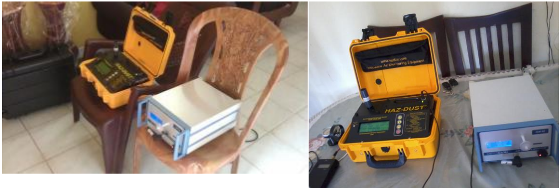
Figure 3-8: Setup of Air Quality Monitor & Haz-Dust EPAM 5000 real-time particulate Monitor
