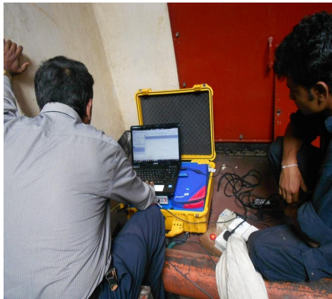
Figure 3.18 Monitoring the waveform along the frequency sweep 'original in color'
