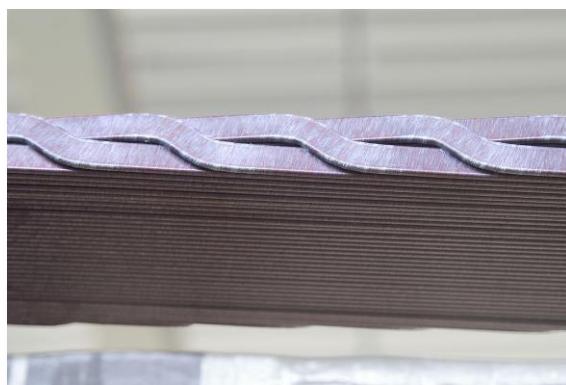
Figure 1.3 : Transposition of roebel bars 'original in color'
