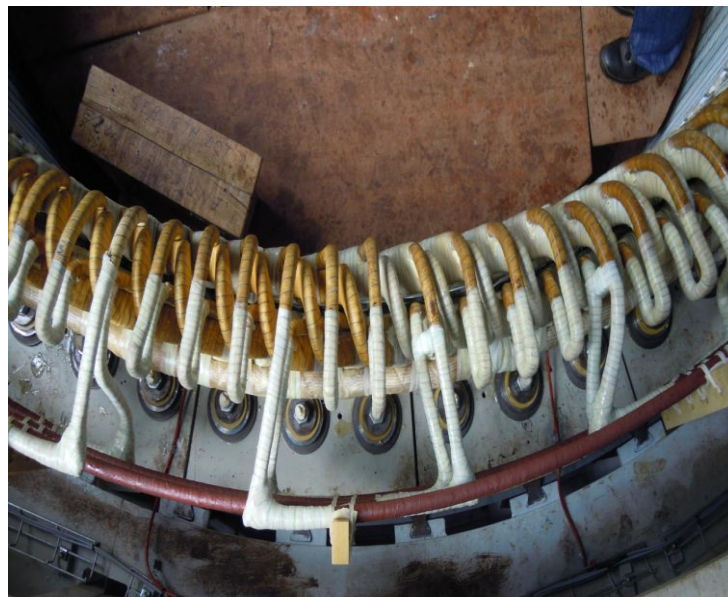
Figure 3.11: Wimalasurendra form wound stator 'original in color'
