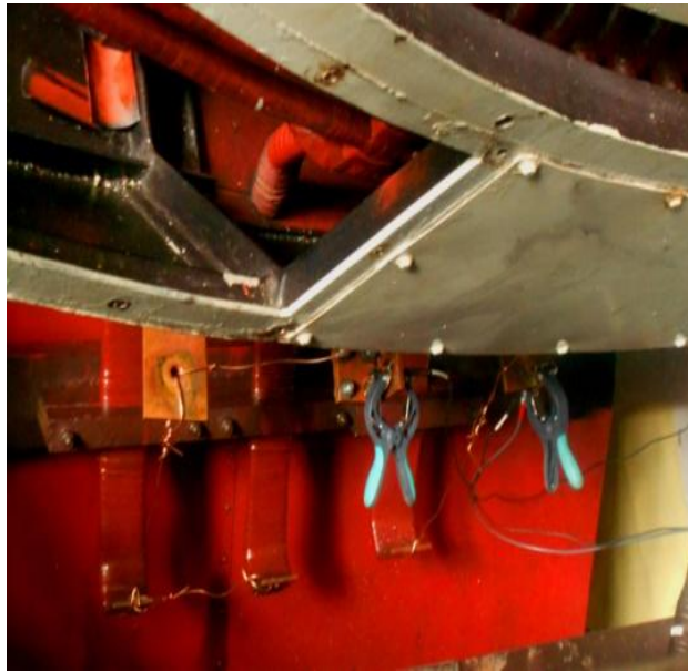
Figure 3.16 : Voltage application to one phase of VPI stator of Old Laxapana while
