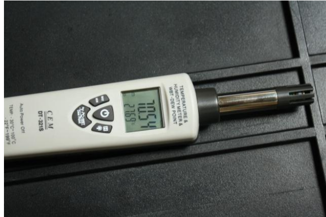
Figure 3.10 : Measurement of temperature and relative humidity 'original in color'
