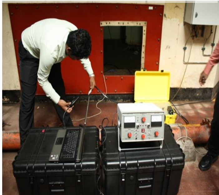
Figure 3.9 : Setting up the apparatus to test GVPI stator 'original in color'
