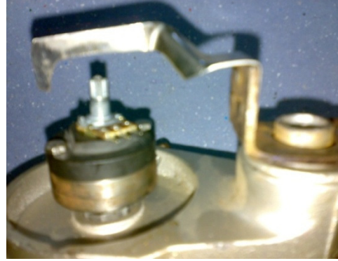
Figure H4: Modified indicator unit fitted to fan belt adjuster
