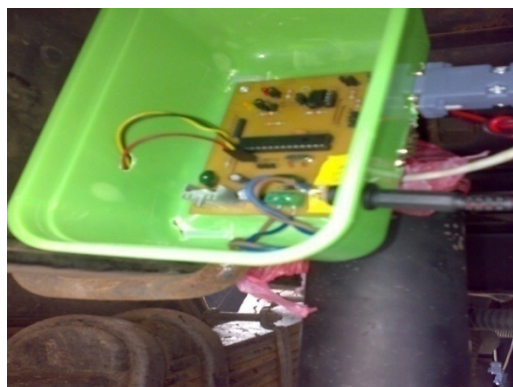
Figure G12, G13: Obtaining values from LSU by loading known weights
