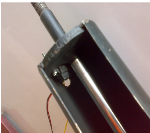
Figure G3: Fitted Infra red sensor
