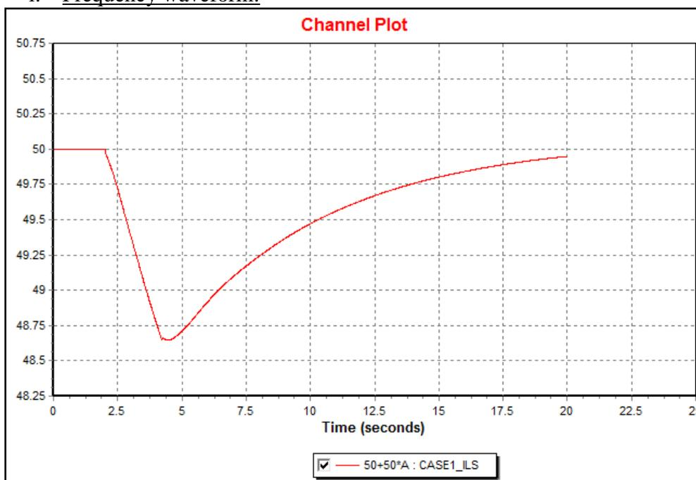
Figure 4.7 Frequency waveform obtained for case study-01
