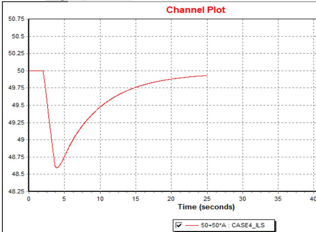
Figure 4.13 Frequency waveform obtained for case study-04
