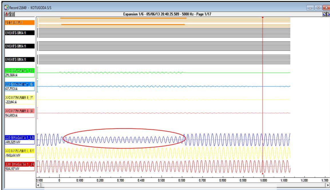
Figure 2.2 DFR record at Kotugoda GSS at 20:41 hrs
