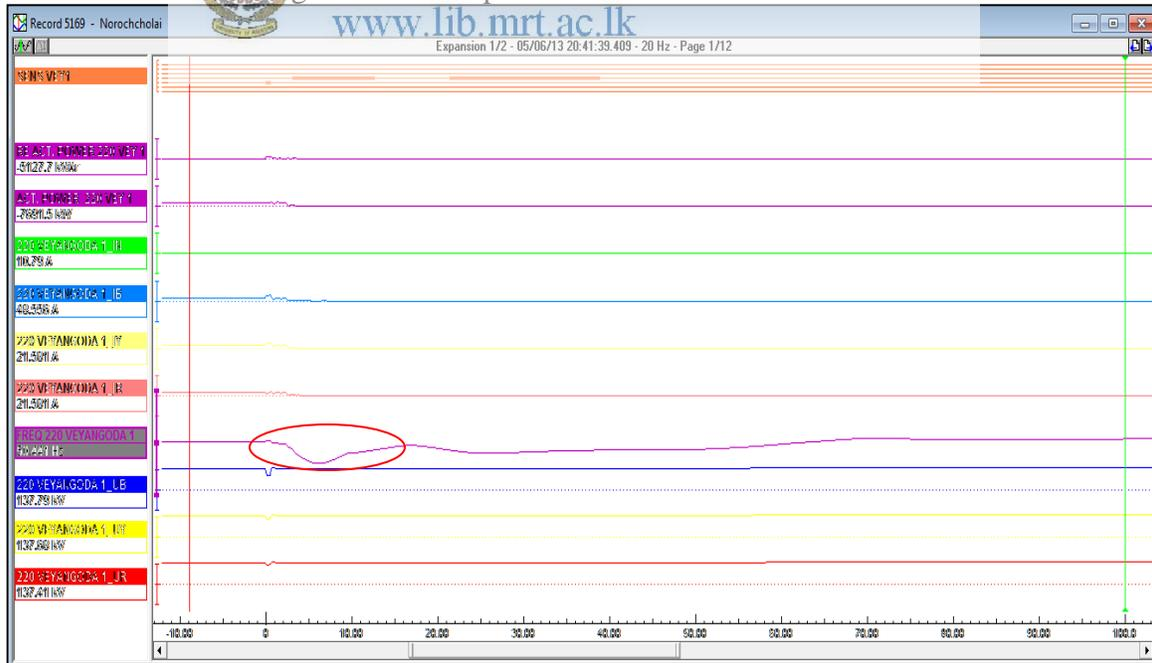
Figure 2.3 DFR record at Lakvijaya power station at 20:41 hrs
