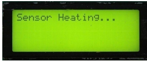
Figure 3.4-d Switching on-chip Heater & Heating SHT11
