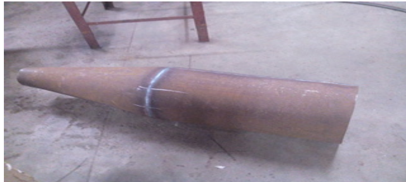
Figure 3.4: Cyclone body Preparation at Workshop
