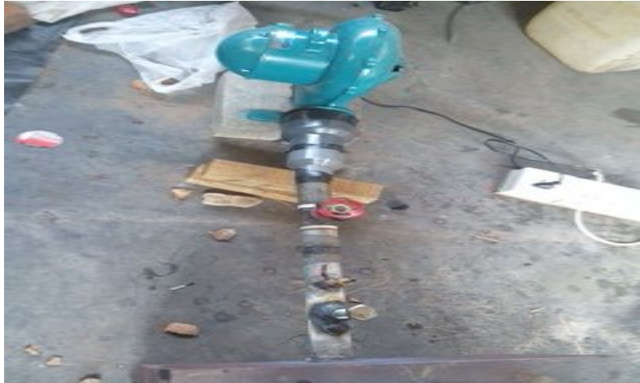
Figure 3.8: Blower and supply line with control valve
