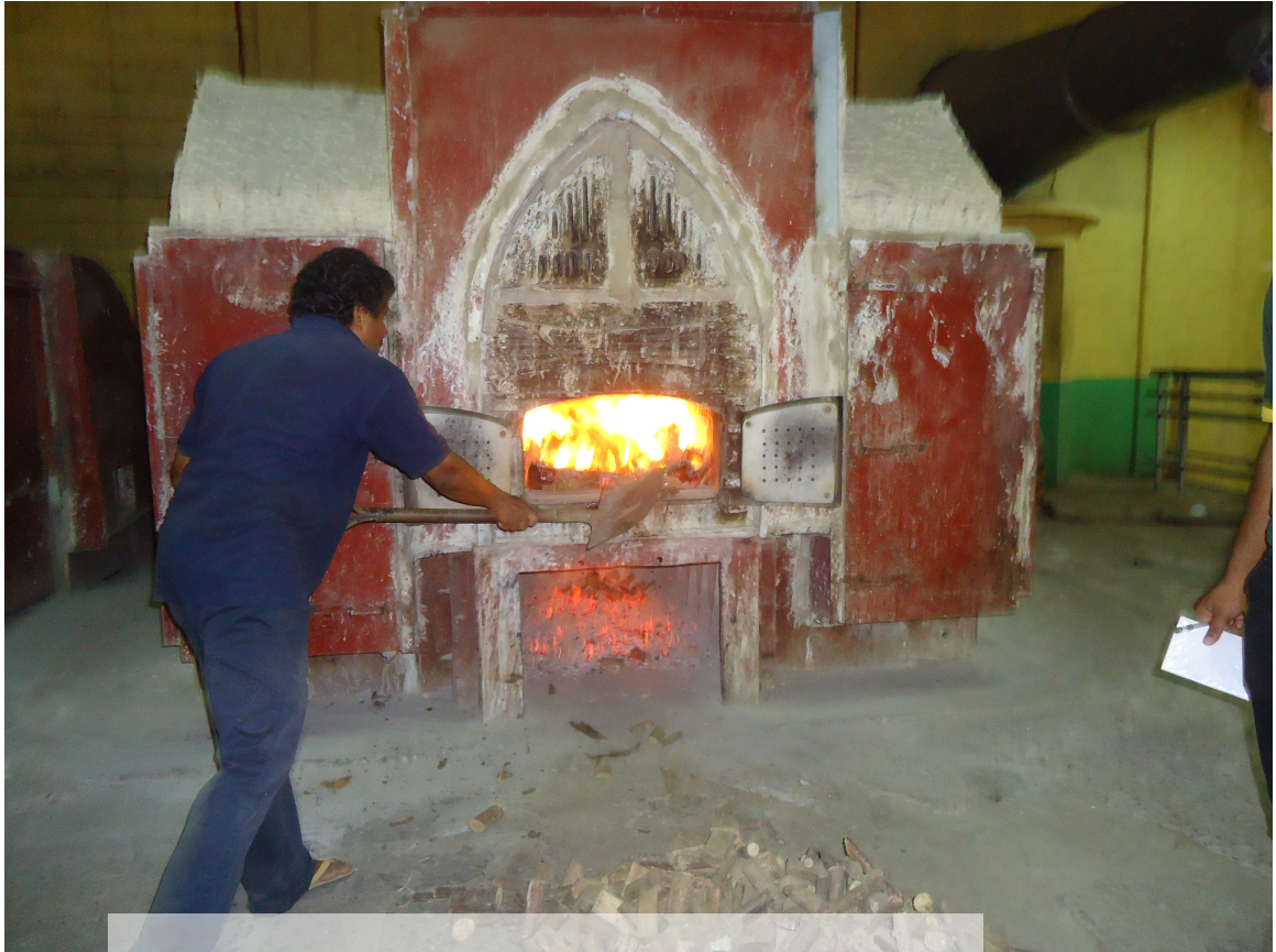
Figure 7.1: Conventional hot air generator system in Tea factories
