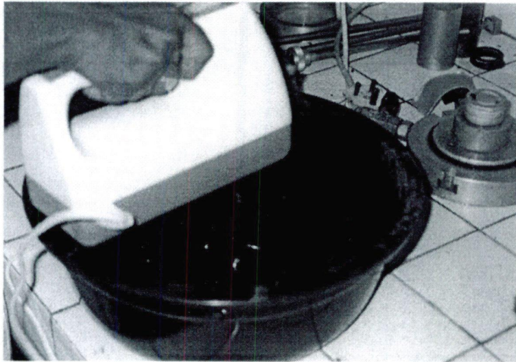
Figure 9: Mixing peat with Cement / Lime using a hand mixer
