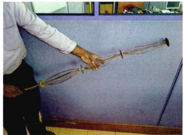
Copper conductor outer strands separated to be laid inside the cylinder – no joints
